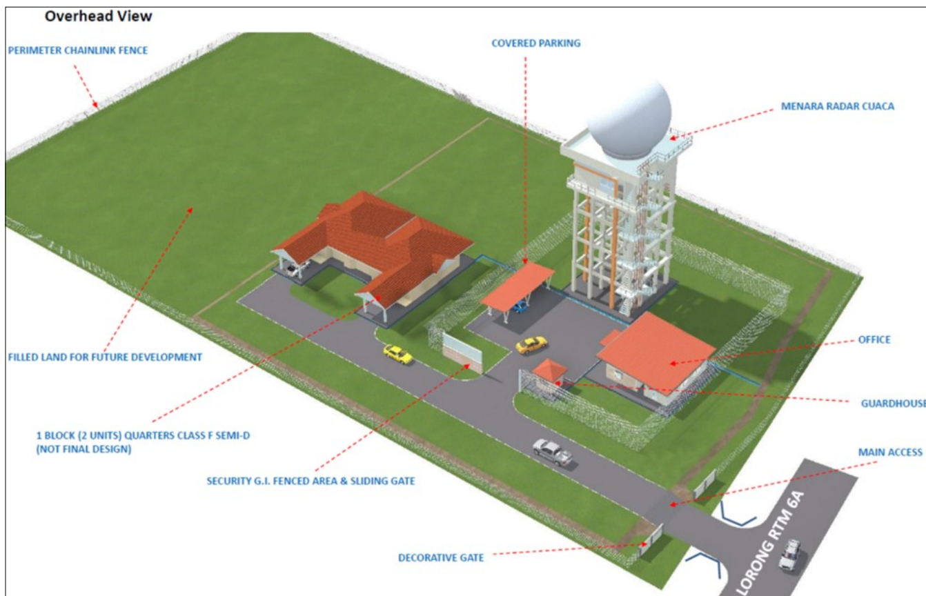
Gambar Illustrasi Pembinaan Stesen Meteorologi Radar Doppler Illustration of proposed construction of Radar Doppler Meteorological Station
